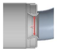
A steel ball with a 28.0mm diameter or solid flat plate measuring 28.0mm and 1.5mm thick must not pass through Section "A" and
