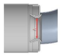
A steel ball with 28.0mm diameter or solid flat plate measuring 28.0mm and 1.5mm thick must not pass through Section "A" and
