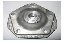
Combustion chamber insert marked 6223387 1 and 6223387 2 must appear as shown below.
